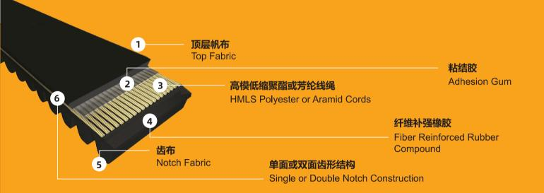
订购代码 Ordering Code 20 X 743 20: 顶宽 Top Width (mm) 743: 节线长度 Pitch Length (mm)
